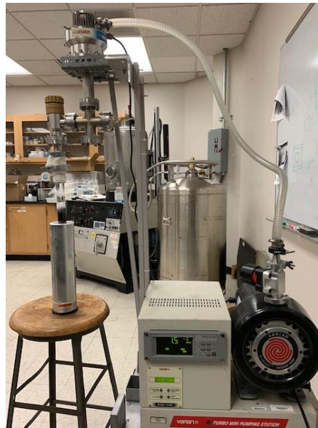
Figure 2.11: Quartz ampoule sealing system at our laboratory for growing crystals.
