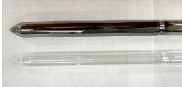
Figure 2.5: Quartz ampoule with carbon coating (top) and without coating (bottom).
