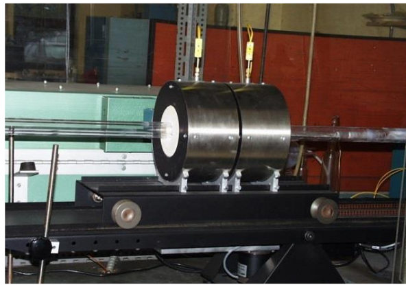
Figure 2.1: In-house horizontal zone-refining system used to purify precursors [38].
